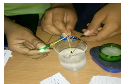
Hands on Activity - Electric Conductivity of Salt Water
